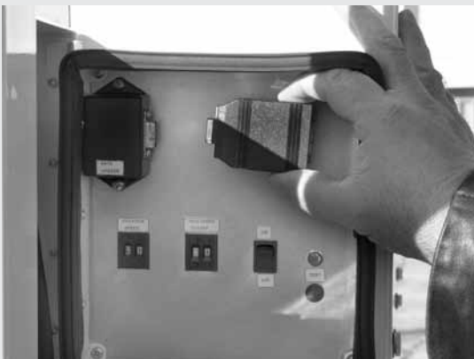
The OnSite 350 is compatible with the EZ Stat™ module, designed to gather speed data samples from Decatur's speed measurement products.
